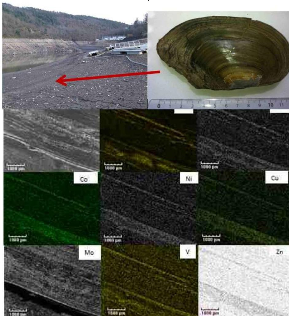
**Figure 4.** SEM image and distribution of heavy metals in shells of freshwater mussels by XR mapping [BILAL, 2013]. Fe, V: yellow, Mn, Mo, Ni: white; Co, Cu: green and Zn: grey.
