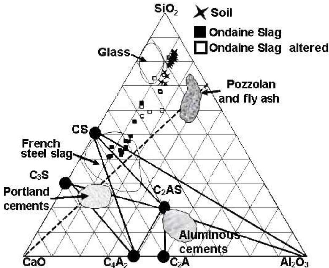
Figure 3. Distribution of slag, altered slag and soil of Ondaine valley in CaO–SiO<sub>2</sub>–Al<sub>2</sub>O<sub>3</sub> diagram. The SiO<sub>2</sub>/Al<sub>2</sub>O<sub>3</sub> ratio is same in slag, altered slag and soil and CaO/SiO<sub>2</sub> ratio decrease substantially. The composition of soil from slag waste is near glass raw material.
